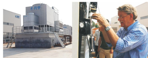
CTI engineers test on Yuanheng cooling tower full performance test platform
