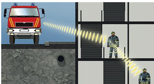
In shielded surroundings the signal of the first alphaSCOUT is extended by the integrated repeater of the second alphaSCOUT.
