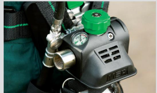
With the filling port fitted on the pressure reducer, all cylinder options can be conveniently filled by a 200 or 300 bar compressor without the need to detach the harness assembly or cylinder.
