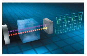
Many gases absorb infrared light at certain wavelengths. The absorption spectrum is distinctive for each gas in question. Infrared Open Path and the Point Technology from MSA use electronically-modulated IR radiation sources at two different wavelengths. One wavelength is typical for the gas to be measured, while there is no infrared absorption by atmospheric gases for the other wavelength.
