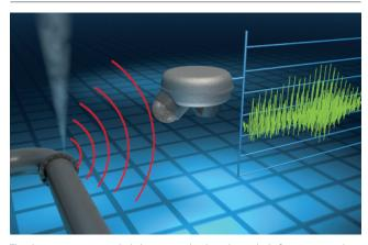
The ultrasonic acoustic gas leak detection technology detects leaks from pressurized gas systems by sensing the airborne ultrasound produced by the escaping gas. This means that the ultrasonic gas leak detectors detect gas leaks at the speed of sound in a detection radius up to 20 meters.
