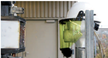
MSA arc flash set before "arc-in-the-box testing" 7 kA
