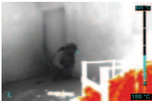
Low Sense Mode: Note wall and ceiling separation
