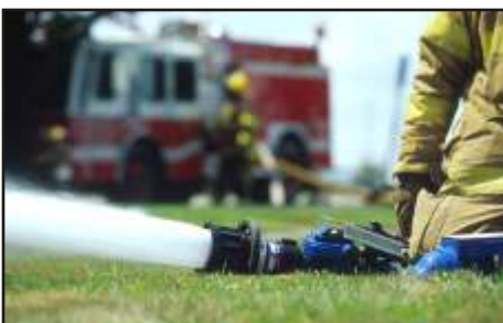
ELEVATION CONTROL - Lifting the nozzle changes the elevation from 10° to 50° instantly.
