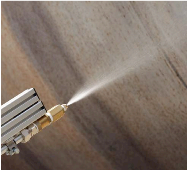
Figure 4: Flat fan nozzle for controlled water dosage
